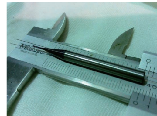
Workpiece R1 cutting tool Size \phi 0.2 x 37mm
