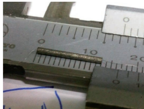
Workpiece tungsten carbide Size \phi 0.1 x 13mm
