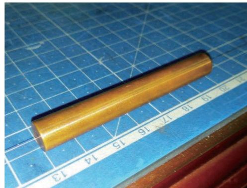
Workpiece OFHC, pure copper Size \phi 0.3 \times 67\text{mm}
